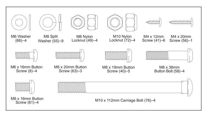
Orient the Rear Stabilizer (16) as shown. While another person lifts the Frame Rail (52), attach the Rear Stabilizer to the Leg (20) with two M10 x 112mm Carriage Bolts (76) and two M10 Nylon Locknuts (72).
